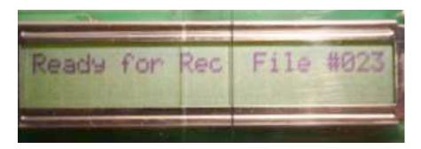
Pressing the RECORD menu button will place the controller in a ready to record state.
