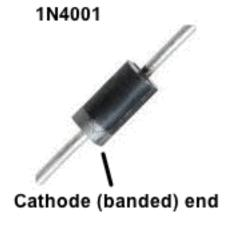
The blocking diodes are a polarized device, and must be installed with banded end toward the V+ (positive) rail of each solenoid. If you are unsure which side is the common positive rail, please contact Resonant Instruments for assistance.
