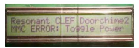
If the card is installed, and repeats the error after the CLEF Controller has been restarted, this indicates the SD memory card has experienced an error. Please contact Resonant Instruments for instructions on replacing the SD memory card.
